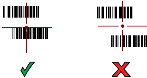
Figure 95 RS6000 Pick List Mode with Multiple Barcodes in Aiming Pattern
